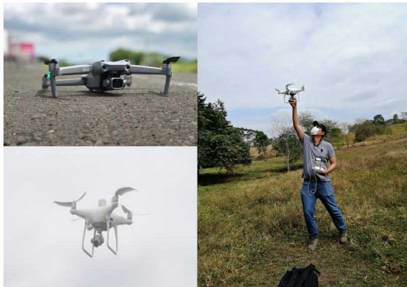
Figure 3. Application of remotely piloted aircraft (drones) to produce aerial orthophotographs and digital elevation models (DEM)
