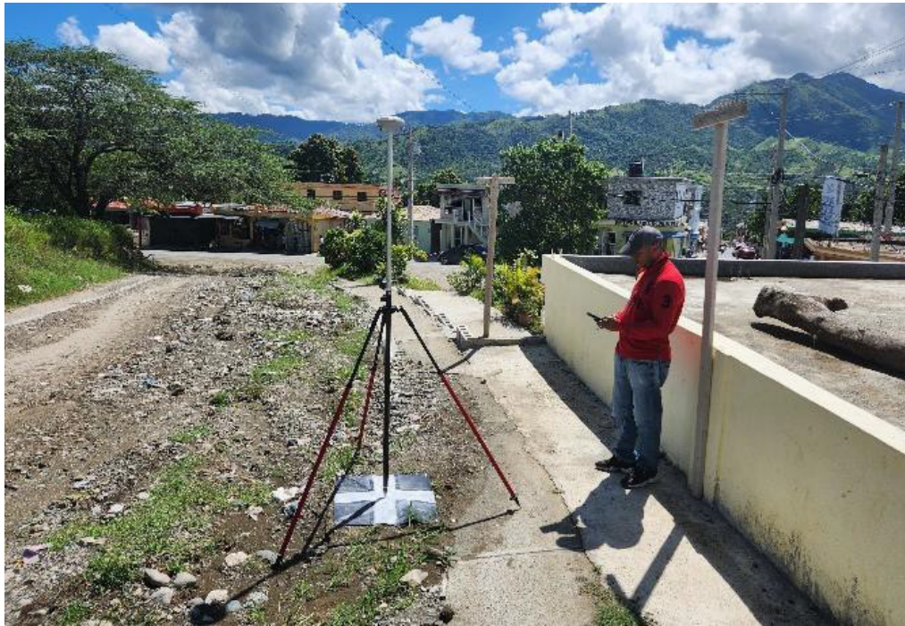
Figure 4. NTRIP Ground Control Point GCP survey is performed
