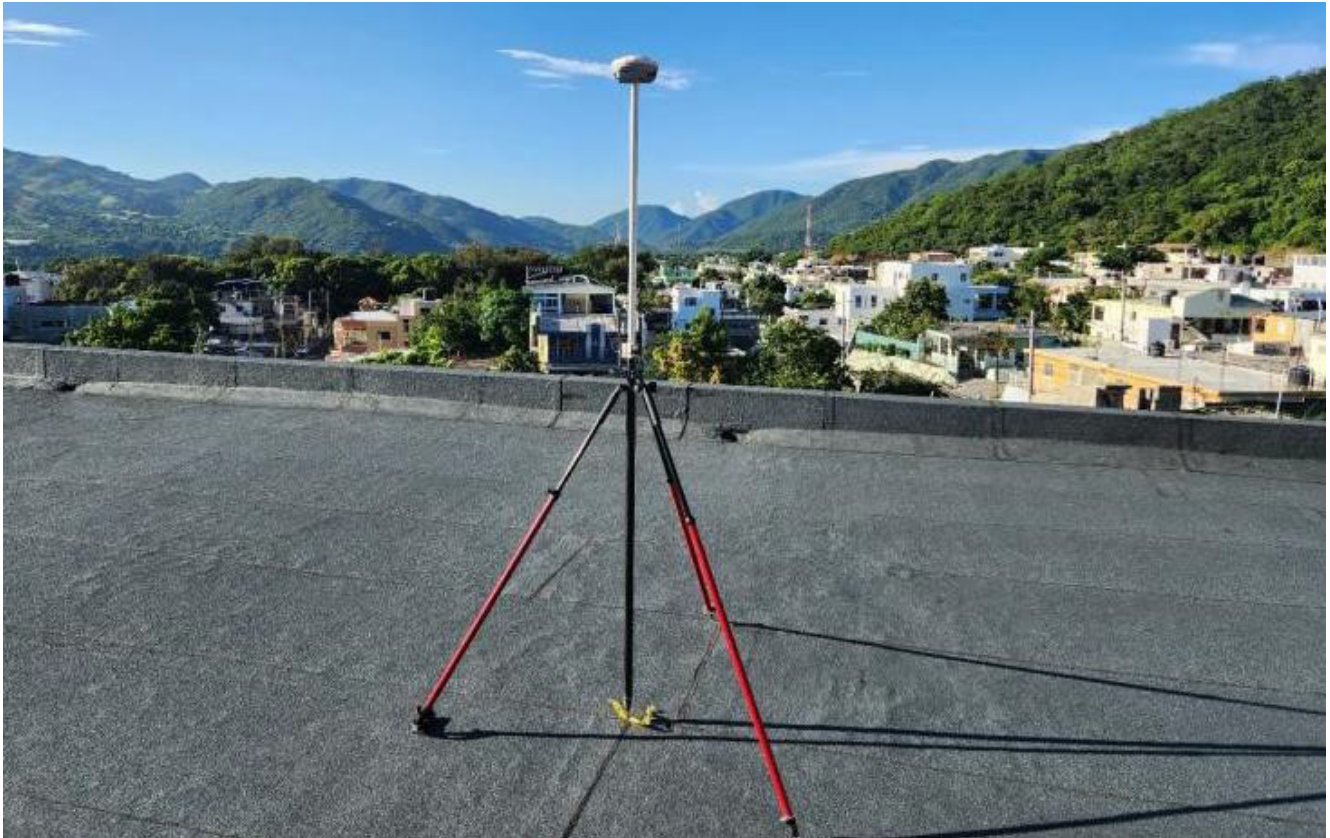
Figure 6. GNSS Receiver at Base Point on the roof of the Altagracia Brito School
